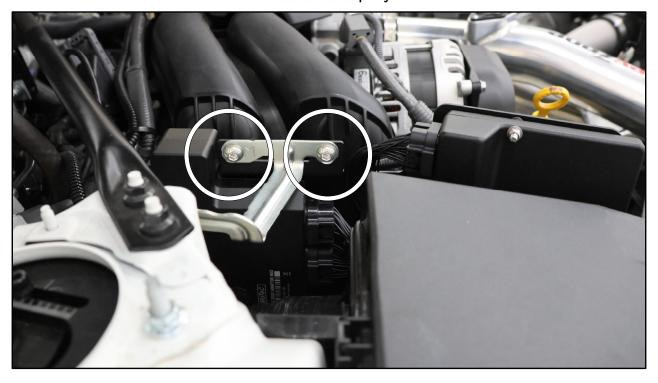
Step #18 Secure Adaptor Kit Assembly using OE Bracket that was removed in Step #3 as shown above using supplied  $2 \times 15 \text{ mm}$  button head bolts (13) with the nuts that were removed in Step #3.
