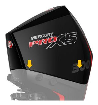
Reinstall the engine cowl as per the instructions under the access panel.
