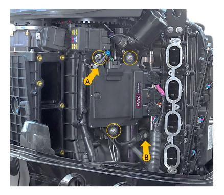
4. Install the 3 x ECU mounting bolts (apply Loctite) & washers (Circled). Torque the bolts to 5Nm.
