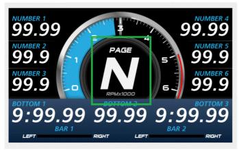
The centre display is normally used to display the current gear but can be used for other purposes.
