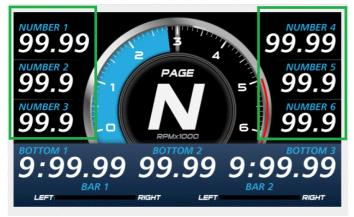
The numeric displays can be programmed to display any channel value.
