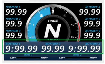
At the bottom, up to 20 lines can be accommodated, with each line containing up to 3 channel values at a time.
