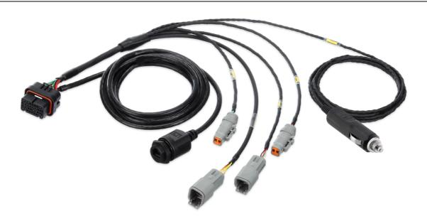
The CDL3 Race Loom enables quick, convenient installation of the CDL3 Track Kit to your vehicle, providing plug-in connection of the CDL3 Dash Logger to power, ethernet, ECU, GPS and buttons. In addition, the loom has an Accessory lead that can be used to connect a MoTeC CAN based product, such as an LTC (Lambda to CAN module), Expander or Video Capture System.
