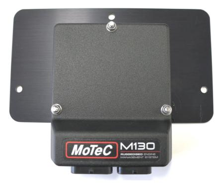
6. Fit the M130 ECU over the 3 mounting studs and secure with M3 x 5mm stainless washers and M3 x 5mm Nylock nuts.
