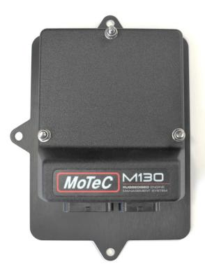
6. Fit the M130 ECU over the 3 mounting studs and secure with M3 x 5mm stainless washers and M3 x 5mm Nylock nuts.
