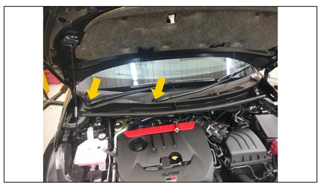
**Step 3: Remove Wiper Components**
