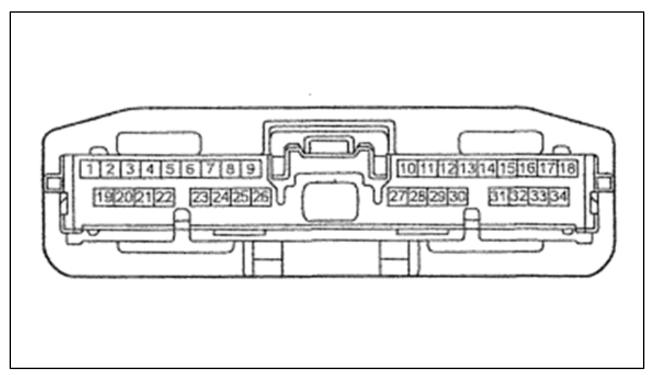
• The CAN bus that needs to be intercepted is on pins 30 (red wire CAN HI) and 29 (white wire CAN LO).
