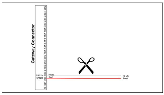
Cut the CAN Hi (red) and CAN Lo (White) wires approx 100 mm from the gateway connector.
