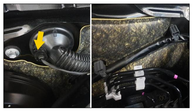
Secure the gateway loom along the factory harness and connect the breakout connector to the adaptor box.
