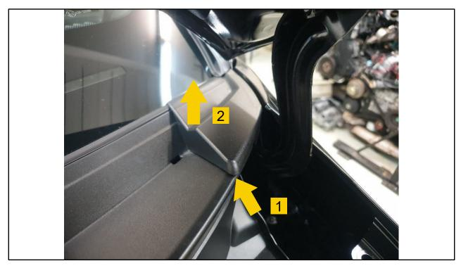
Remove the corner capping pieces from the wiper tray cover.
