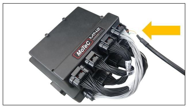
When fitting the stub loom with the Ethernet communications cable, plug the end
