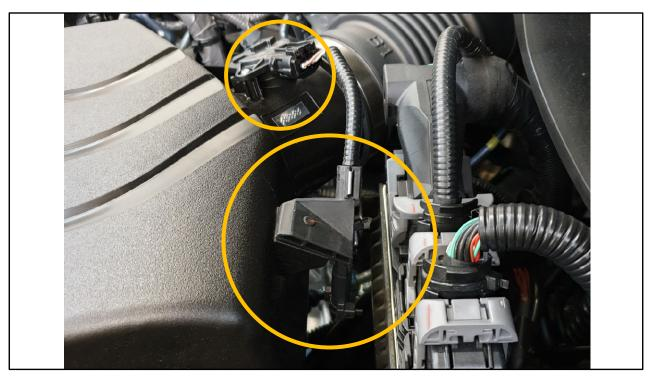
Unclip the wiring support bracket from the airbox lid
