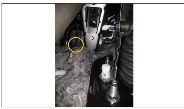
• From inside the driver's footwell area, secure your gateway loom to your pull aid. The CAN wires need to be secured to the pull aid, and then pull the wiring through the firewall grommet carefully, ensuring the loom does not get caught on anything or wrapped around any pedals. This is easiest with one person guiding the loom, whilst another person pulls it through. (note in the image, the gateway loom has already been pulled through).
