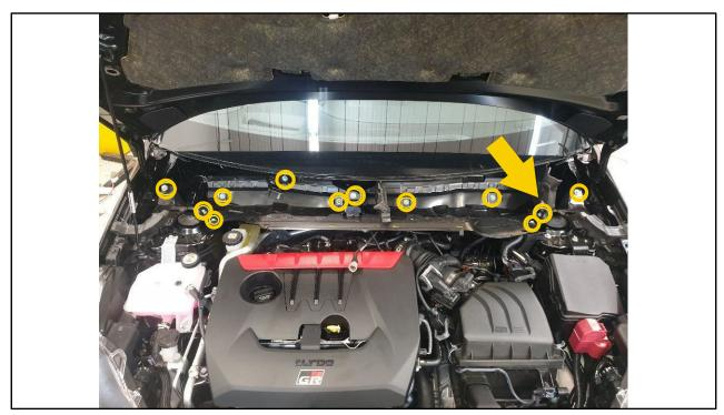
Unbolt the lower wiper cowl by removing the 12 x M6 bolts.
