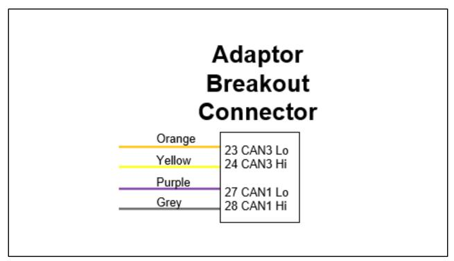
Connect the 4 terminated breakout loom wires to the Adaptor Breakout Connector as shown. See also loom schematic.
