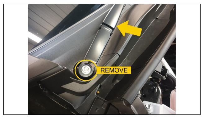
Once the wiper bolt is removed, remove the wiper arm by applying and releasing pressure
