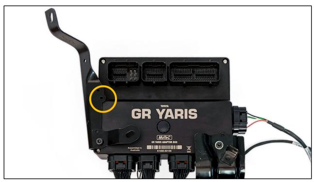
Drill out the hole (as marked) on the OE ECU bracket to 5 mm.
