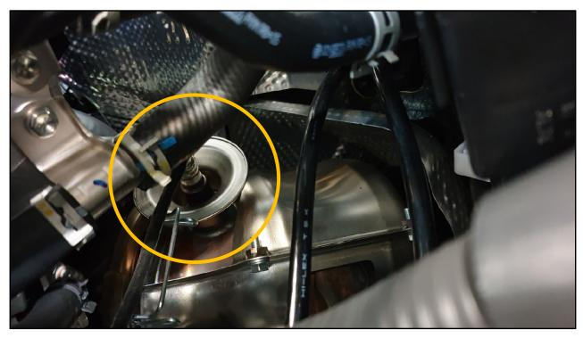
With the sensor wiring unhooked, fit a Lambda sensor socket onto the sensor, as well as a universal joint.
