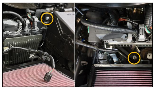
• Remove the highlighted nuts and bolts using the 10mm socket, extension and ratchet.
