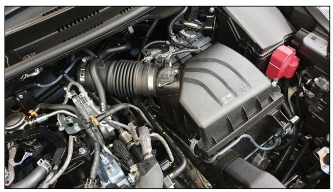
Refit the upper airbox in the reverse method to the removal procedure.
