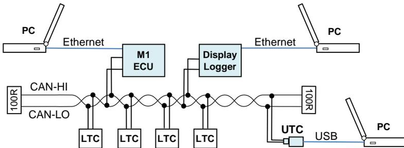
The gateway device must be selected in LTC Manager as shown below. For gateway devices that have multiple CAN interfaces (e.g. Display Loggers), the appropriate CAN bus must also be selected.
