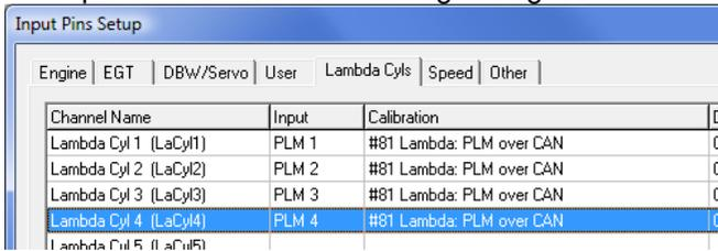
**Assign Lambda measurements to a M84 channel**
