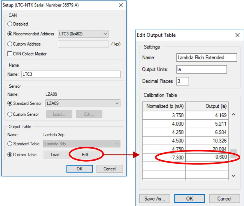
At the lower end of the table, users can enter their own values for richer mixtures. The table will be reordered when **Enter** is pressed.
