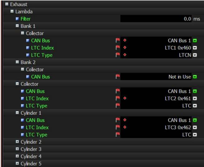
LTC devices are configured in M1 Tune by setting the CAN bus, Index and LTC Type.
