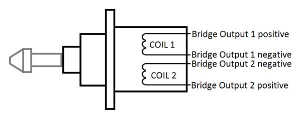
Determining how the coils are wired is a simple matter of using a multimeter to find the pin pairs that have the same resistance. On a GM style stepper motor, coil 1 and coil 2 will have the same resistance and there will be no connection between the two coils.
