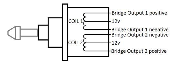
The 12v connection is not essential to the operation of the stepper motor as the MoTeC outputs are full bridge outputs and can switch both high side and low side. If the stepper motor has six pins, however, it is recommended that they be connected to the 12V+ ECU Supply.
