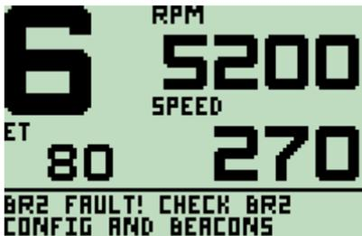
Note that this condition only applies for the first invalid beacon found after a valid beacon or after power up. The fault message indicates that either the BR2 is not configured correctly for the MDD and for the beacon transmitter being used, or that the beacon transmitter is incorrectly configured, faulty or missing.
