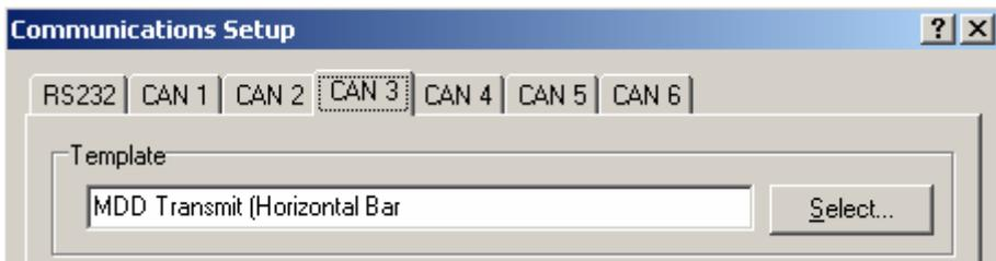
The second template contains the channels to be sent. While these can be configured by the user, included with Dash Manager is a template that contains 8 Exhaust Gas Temperature channels. For this option, choose a second (blank) CAN tab and select the comms template 'MDD Transmit (8 x EGT)'
