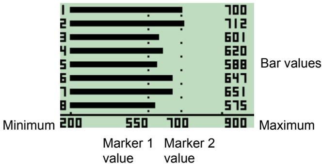
The eight bar graph values and the two marker positions are scaled according to the Maximum and Minimum values received from the ADL, within a range of -999 to 9999.
