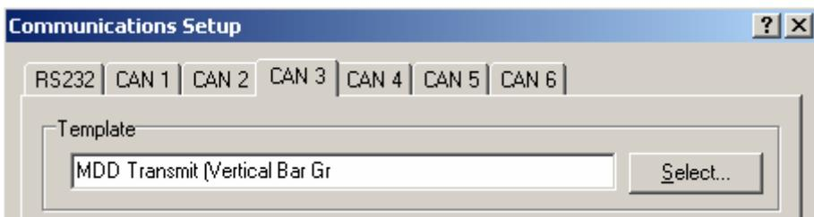
The second template contains the channels to be sent. While these can be configured by the user, included with Dash Manager is a template that contains 8 Exhaust Gas Temperature channels. For this option, choose a second (blank) CAN tab and select the comms template 'MDD Transmit (8 x EGT)'
