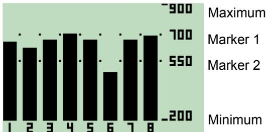
The eight bar graph values and the two marker positions are scaled according to the Maximum and Minimum values received from the ADL, within a range of -999 to 9999.
