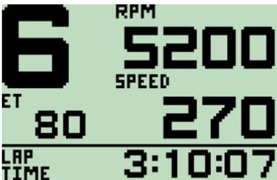
The most recent lap time and fastest lap time can be displayed at any time by scrolling to the appropriate User Mode layouts with the button. Lap time and fastest lap time are reset on MDD power up, and if communication to the BR2
