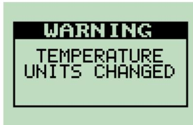
The current temperature mode is stored in the MDD, and may be viewed in the MDD INFORMATION screen in tuning mode. When powered up the MDD will use the mode last set.
