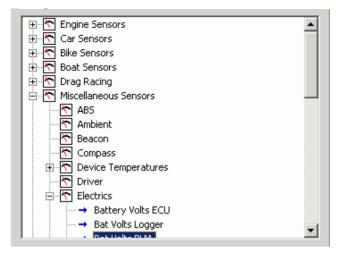
A Tree Structure is used to select items from a hierarchical list The UP ARROW key moves the cursor up (selects the item above) The DOWN ARROW key moves the cursor down (selects the item below) The RIGHT ARROW key expands; expandable branches indicated by a plus sign (+)
