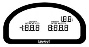
The three numeric displays–left, right and top right–can be programmed to display any value, which may be different for each of the display modes (Warm-up, Practice and Race).
