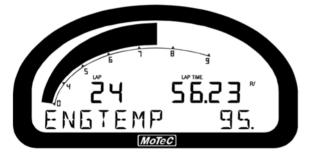
The alarms remain active until they are acknowledged, either by a driver activated switch or automatically after a defined period of time.
