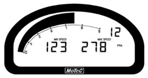
The Practice display is used to display basic information, plus information to help the driver improve lap times, e.g. Lap Time, Lap Gain/Loss, Maximum Straight Speed, Minimum Corner Speed or Corner Exit Speed.
