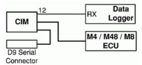
Contact MoTeC for the CIM module drawing for full wiring details.
