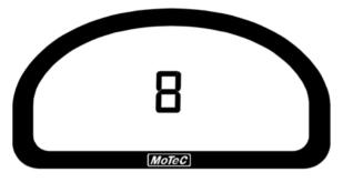
The centre numeric display is normally used to display the current gear but can be used for other purposes.
