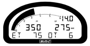
The Warm-up display is used to display important engine sensor readings during engine warm-up, e.g. RPM, Battery Voltage, Engine Temperature, Oil Pressure, Oil Temperature and Fuel Pressure.
