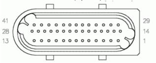
Looking into the plugs on the adapter loom
