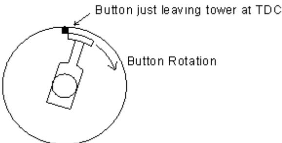
The button must be a wide tip type to cater for a wide range of advance points since the advance is changed electronically rather than mechanically.
